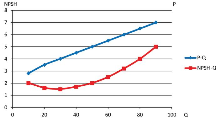
In addition to head, the power consumption (P) is also to be found in the data sheet. The power consumption is used for dimensioning of the installations which must supply the pump with energy. The power consumption is like the head shown as a function of the flow.
